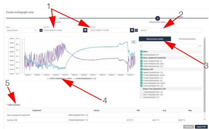
Figure 164. Smart-Vue Pro web application of multigraph display
