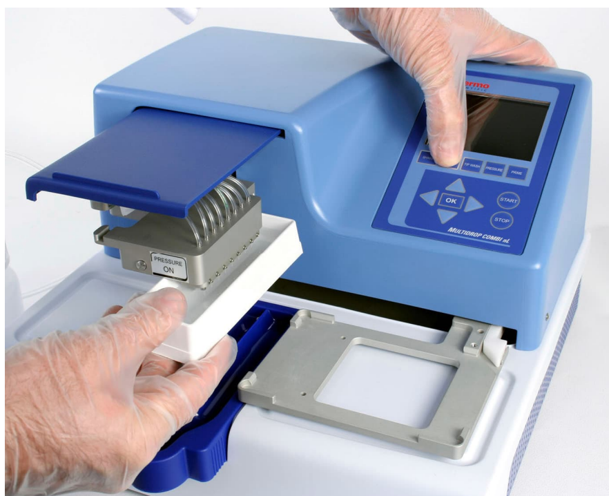
Figure 5-24. Cleaning the tubings using a reagent basin
