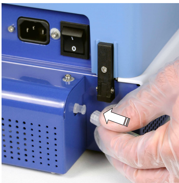
Figure 3–10. Connecting the hosing to the pressure/vacuum system
