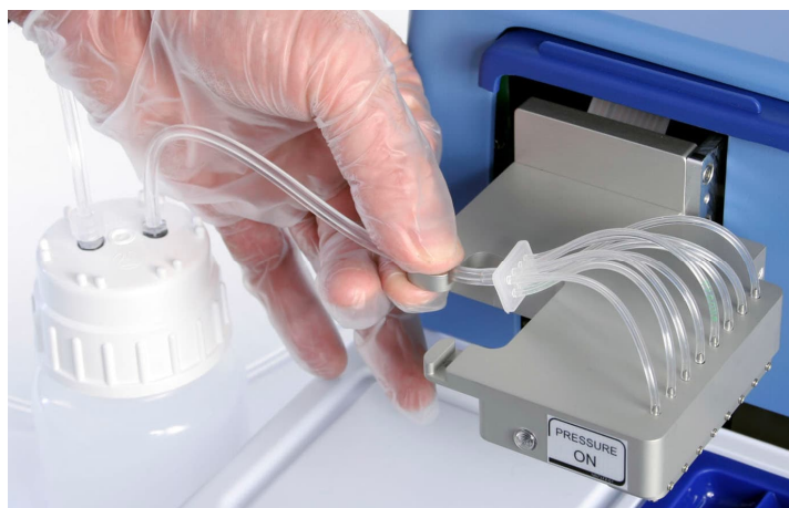
Figure 5–31. Replacing the tubing set and manifold
