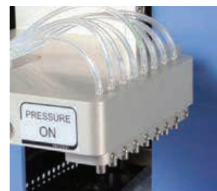
Figure 2. Eight dispensing valves inserted into the manifold.
