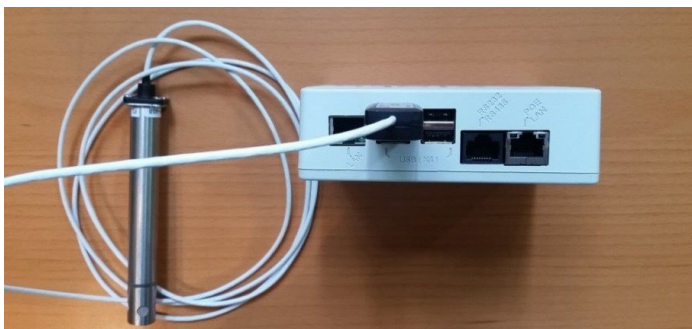
Figure 1. Sensor connected to USB port
