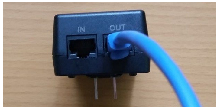
Figure 4. Ethernet cable connected to PoE injector from mote's PoE/LAN port
