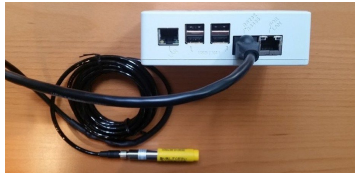
Figure 2. Sensor connected to RS232/RS485 port
