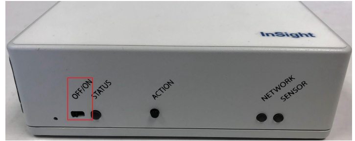
Figure 6. Mote OFF/ON switch
