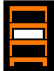
Figure 27. Unit Selector Display – Middle LED Selected (PRO model)
