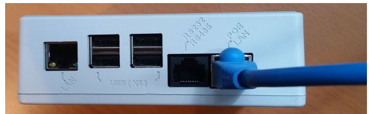
Figure 3. Ethernet cable connected to PoE/LAN port from PoE injector, PoE switch, or PoE-enabled outlet
