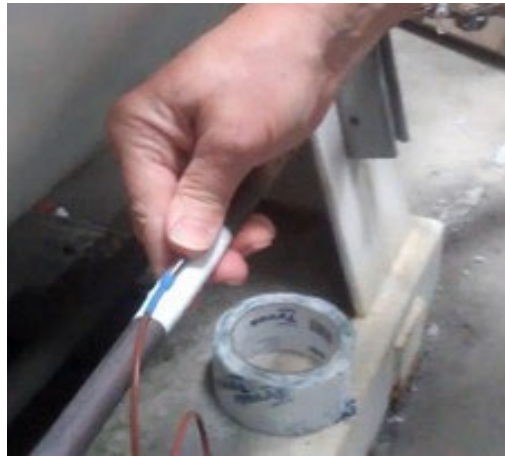
Figure 45. Center RTD sensor on Teflon tape
