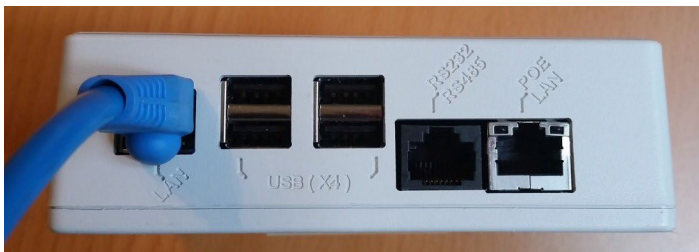
Figure 5. Ethernet cable from computer connected to LAN port
