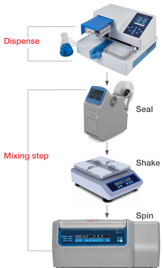
Figure 1. The high-throughput Multidrop Combi+ Reagent Dispenser workflow. In the revised workflow, the Multidrop Combi+ dispenser replaces the aspiration and dispense step. In the mixing step, a pipette is replaced by sealing the microplate, shaking for ~30 seconds, and spinning for ~30 seconds. With the dispensing speed of the Multidrop Combi+ dispenser and the 4 plate positions of the Thermo Scientific™ Digital Microplate Shaker, labs can process 4 plates per reagent faster than it would take using an ALH.
