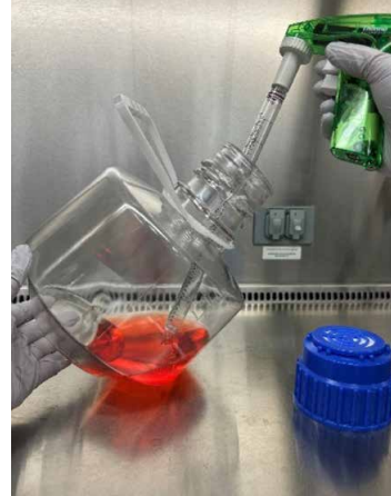
Figure 3. Example of a 5 L shake flask undergoing a 50% medium exchange.
